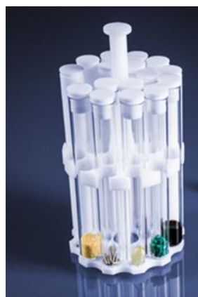
Fig. 4: The digestions were performed with Pressure Sealed Vials in Rack 18
